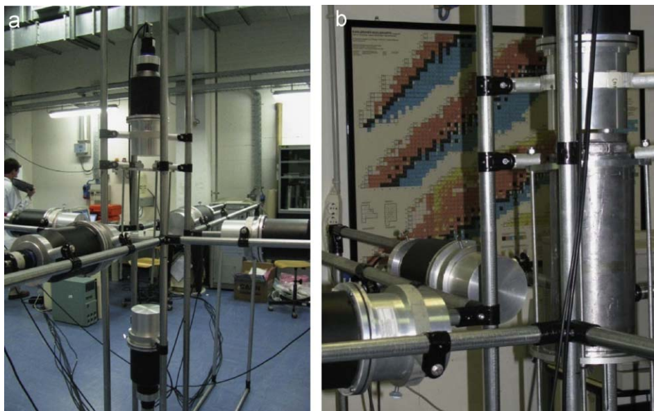
Fig. 1. Photographs of the measurement setup showing: (a) six EJ-309 liquid scintillators and centrally located ^{252}\text{Cf} source and (b) plutonium-oxide sample shielded by lead sleeves of thickness approximately 2.6 cm.
